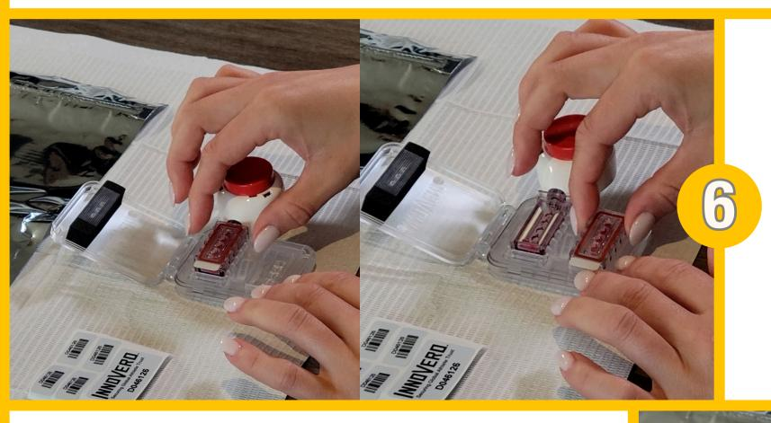
To seal the sample, the athlete opens the InnoVero DBS security kit, keeping the piece of black foam at the top. The plastic cartridge that houses the four collection pods is placed in the grooved upper compartment. With a finger on top of the cartridge, the athlete pushes down on the device with their other hand to remove the cartridge. The athlete moves the cartridge to the lower compartment of the case.
